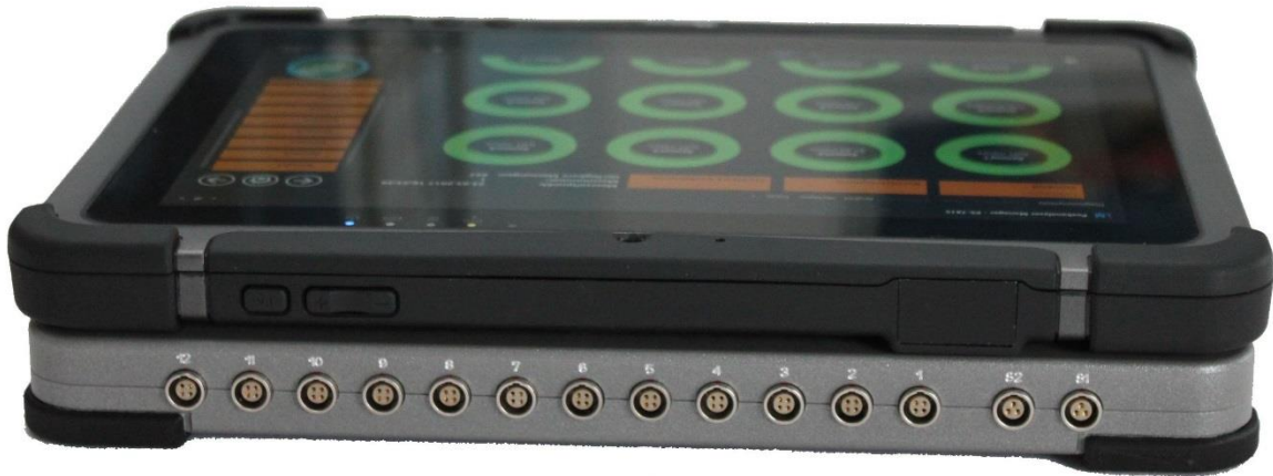
Picture 4: Sensor inputs on upper side
